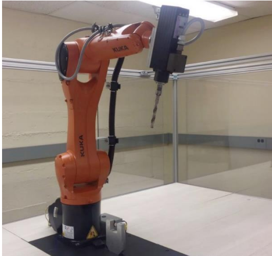
Fig. 3. KUKA robot with spindle installed.
